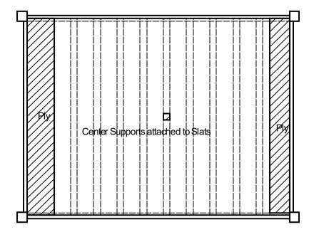
Secure all slats and plywood slats with screws provided.
